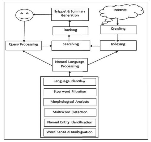
Figure 1. IR System Architecture
